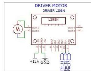
Gambar 6. Rangkaian driver motor dan motor DC
